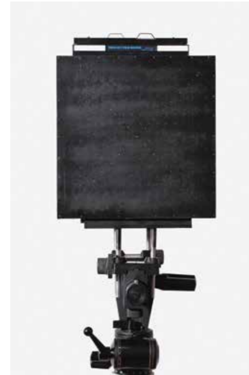
Divide Genius II Felix Frühauf, 2018 Sinar camera with camera obscura grid through which approximately 200 small images were simultaneously projected onto a 8 × 10 inch b/w film Courtesy of the artist
